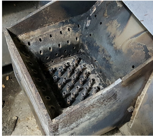
Fig. 4. Modified burner with the nozzle-type burner pins.
