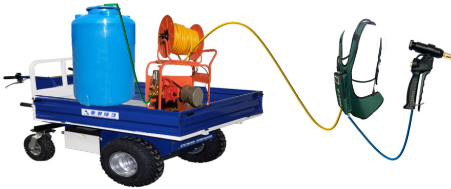
Fig. 1. Construction of pulsatory direct water spray gun system.
